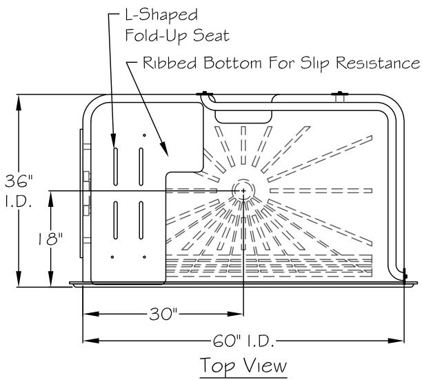
THIS DRAWING IS FOR SUBMITTAL PURPOSES ONLY. THIS DRAWINGS SHOULD NOT BE USED FOR INSTALLATION OF THIS UNIT. REFER TO AQUA BATH'S INSTALLATION INSTRUCTIONS FOR FRAMING AND ROUGH-IN DIMENSIONS.
