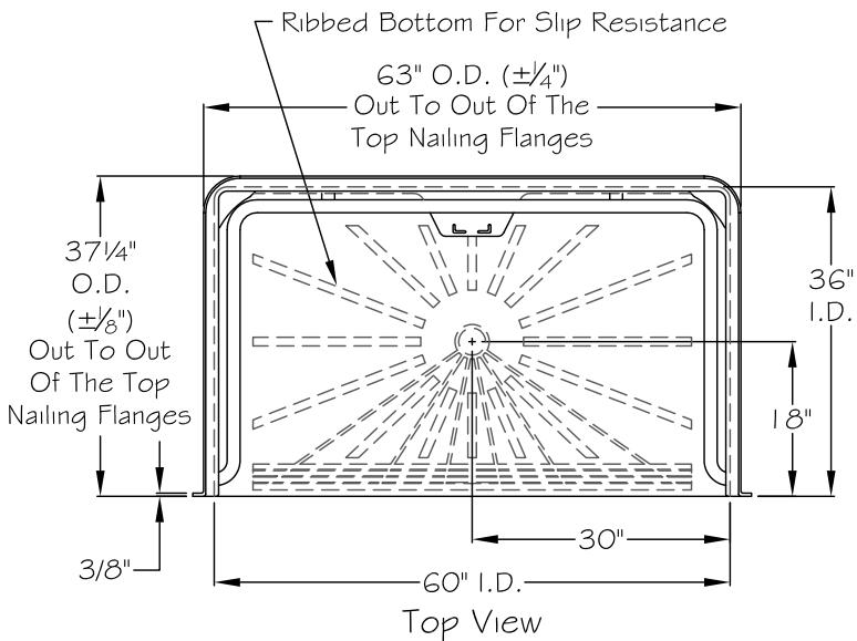
THIS DRAWING IS FOR SUBMITTAL PURPOSES ONLY. THIS DRAWINGS SHOULD NOT BE USED FOR INSTALLATION OF THIS UNIT. REFER TO AQUA BATH'S INSTALLATION INSTRUCTIONS FOR FRAMING AND ROUGH-IN DIMENSIONS.
